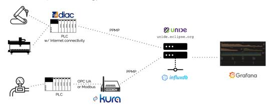
**Eclipse 4diac** is an open source PLC environment that allows to implement industrial control solutions in a vendor neutral way according to IEC 61499 extending IEC 61131-3.
