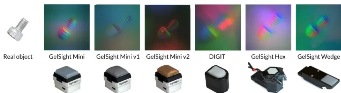
Figure 1: Vision-based tactile sensors vary in both optical design and physical properties. Even with the same contact object, a screw, the tactile images produced by each sensor differ significantly. These variations highlight the challenge of transferring models from one sensor to another.
