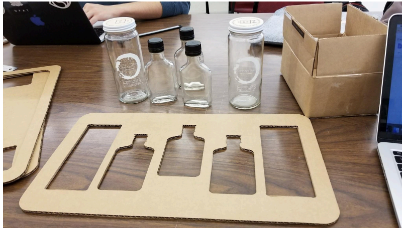
Figure 5: Placement of glass bottles in prototype
