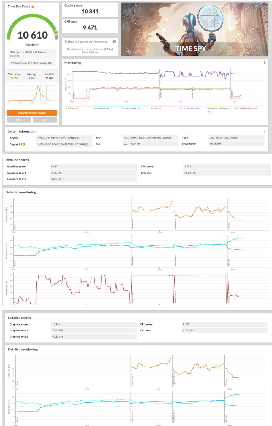
Time spy graphics performance mode Optimus disabled with Overclocking (+150 Mhz Core Clock + 300 Mhz Memory Clock) :
