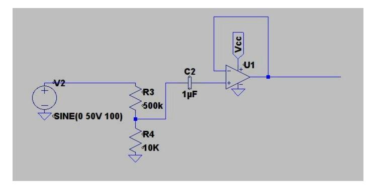
but instead of 500k resistance you have to use a linear potentiometer, it's just a row schem, but it should work :) Vcc is 3.3V
