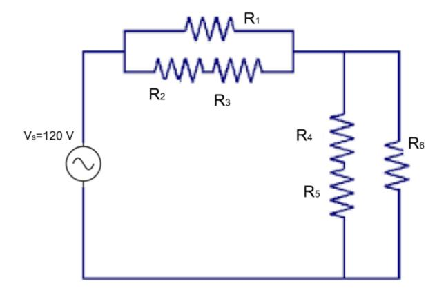
For the following schematic above, fill in the table that describes the flow of electricity through the pathway. Show all of your work on a **separate piece of paper**. It may be useful to make a reduced schematic diagram. *Hint:* to help get you started, make a reduced schematic diagram and put R2 and R3 together in series. After that, make a second reduced diagram and make resistor R123.
