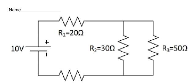
For the following schematic above, fill in the table that describes the flow of electricity through the pathway. **Show all of your work on a separate piece of paper**. It may be useful to make a reduced schematic diagram. *Hint: to help get you started, find the equivalent resistance for R2 & R3*
