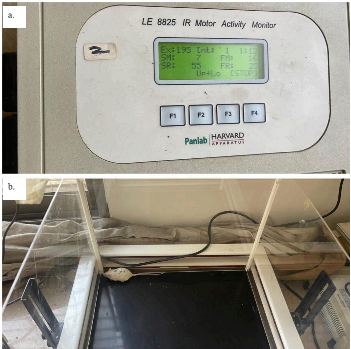
Figure 9 a. Motor activity monitor used to assess locomotion, detecting SM/FM and SR/FR readings; b. An open-field test conducted for anxiety
