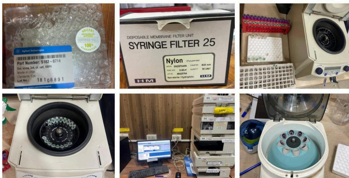
Figure 7 Laboratory equipment and materials used for High-Performance Liquid Chromatography (HPLC) analysis, including Agilent-certified vials, syringe filters, centrifuges with samples, and an HPLC system setup.
