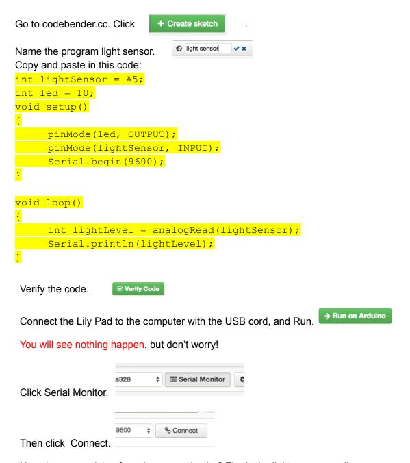
Now do you see lots of numbers zooming by? That's the light sensor reading. Cover the sensor with your hand and watch the numbers change! Do they go down or up? Troubleshooting: If you only see the number 1023, that means your light sensor is not connected properly. Look back at the circuit diagram and check your wiring.
