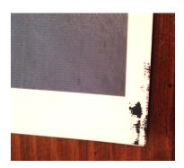
Head strike - If the print head collides with the paper it can leave a big ink mark. This is most common on the edge of the paper but can happen anywhere, especially with curled paper or transparency.
