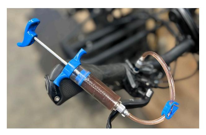
Hydraulic brake fluid (mineral oil and very dirty!) Don't forget to get your brakes bled at least twice a year to keep the power and modulation in top form
