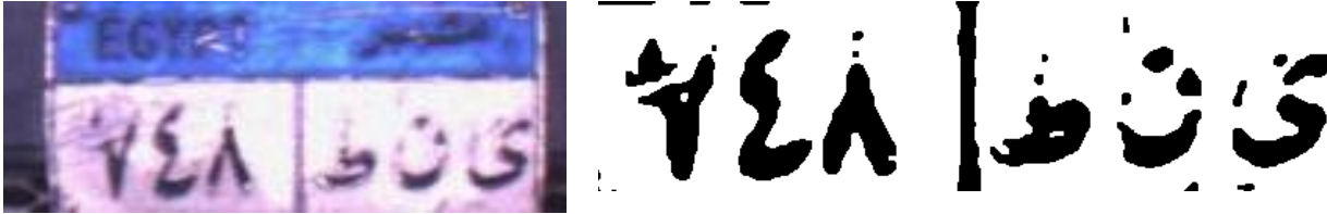
Figure 4.5 Partially erased characters before and after opening and closing operations.
