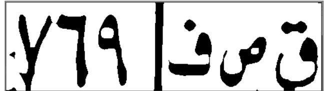
Figure 4.7(c) Blur, Threshold, Dilation and binarization
