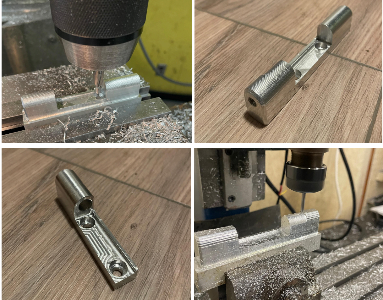
Figure 30: Machining process of the lower hinge component. Multiple 3D CAM programs and setups were used to create the eccentric part.
