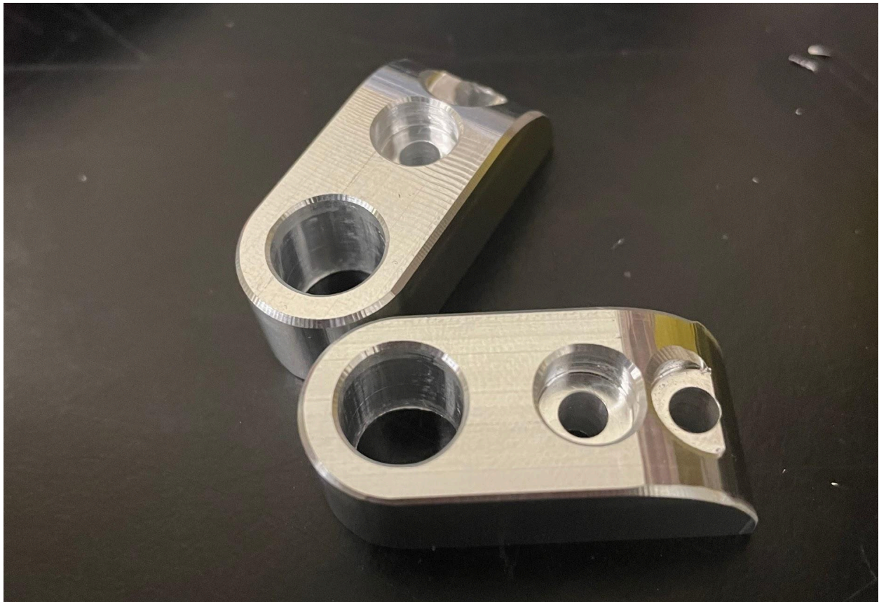
Figure 38: CNC machined locking mech mounts. Bolts to armrest plates via two M4 bolts.
