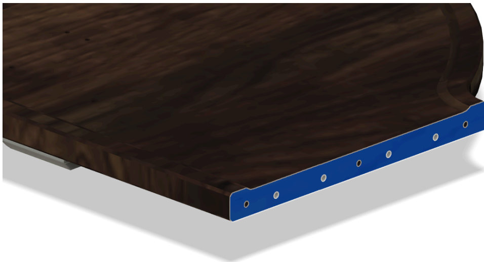
Figure 28: Hinge mounting points. Four M4 bolts and three \frac{1}{8}'' dowel pins.
