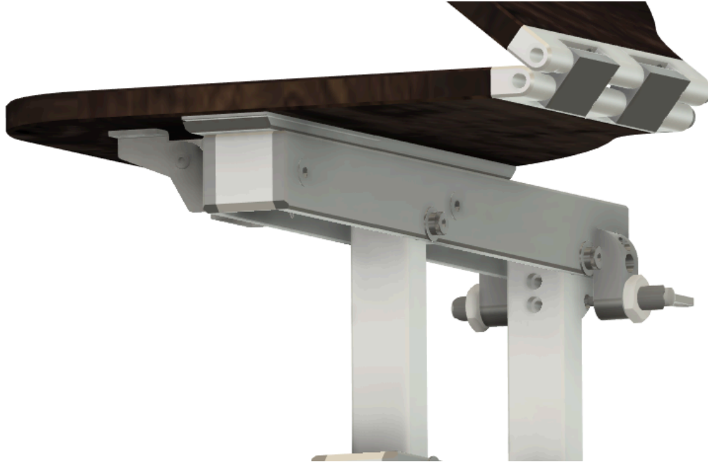
Figure 32: Plasma cut 1/4" aluminum plates make up the structural part of the armrest and the spacer for the desktop to sit square to the armrest.
