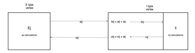
Implementation of this algorithm needs three types of vertices E, I and S. S vertices functionality is containing and sending similarities and this can be done in one of the two vertices, this implementation will use I vertex to do it. This way I nodes will calculate  $\rho ij$  (s(i, j)+ $\eta ij$ ) and  $\beta ij$  (s(i, j)+ $\alpha ij$ ) messages simulating S vertices and avoiding the need of having them in the implementation.
