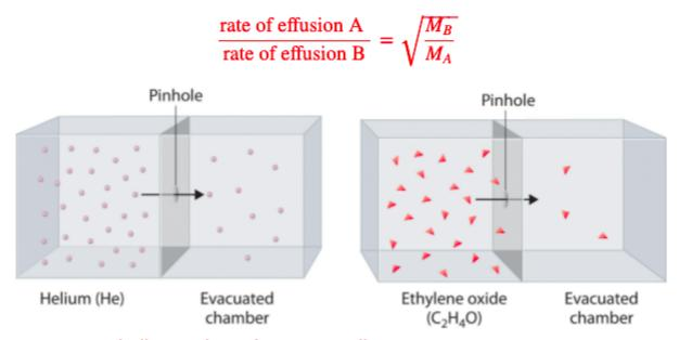
The Relative Rates of Effusion of Two Gases with Different Masses. The lighter He atoms (M = 4.00 g/mol) effuse through the small hole more rapidly than the heavier ethylene oxide (C2H4O) molecules (M = 44.0 g/mol), as predicted by Graham's law.
