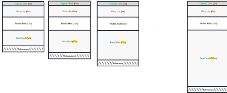
Fig. 4. Site profile models considered to account for the depth to engineering bedrock
