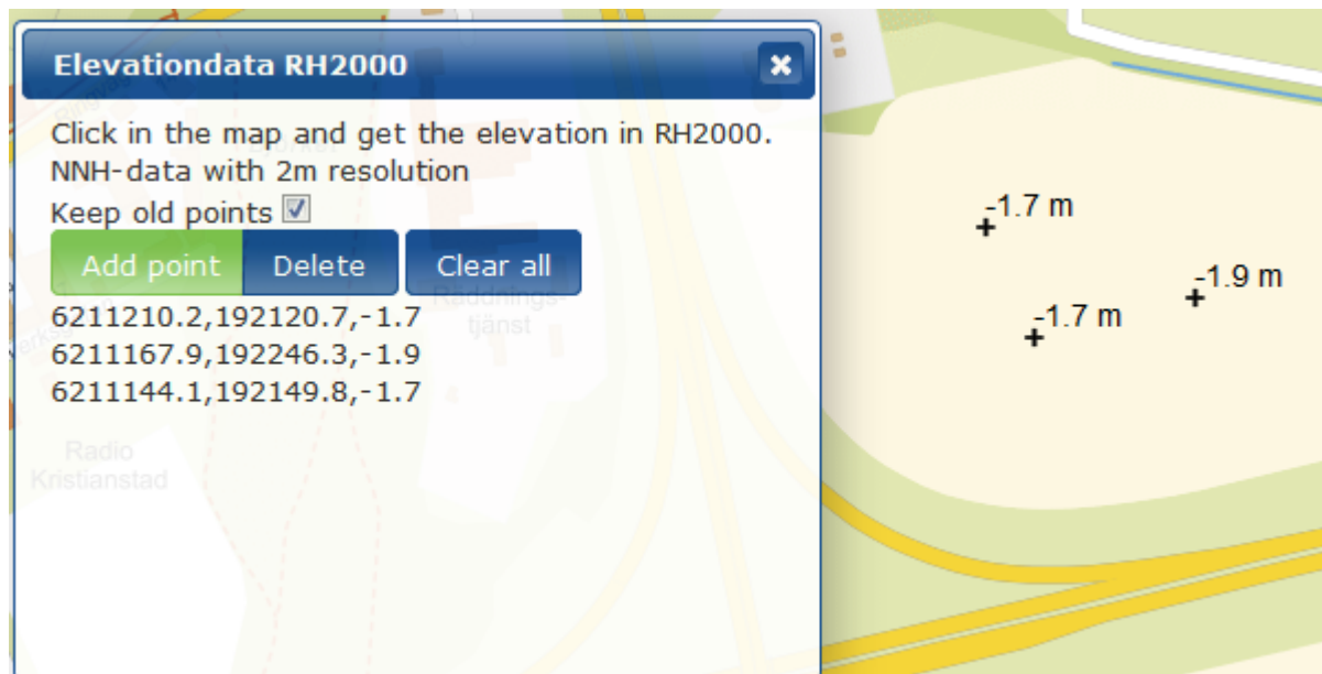
Fig. xx Example of measuring a ground elevation (City of Kristianstad)
