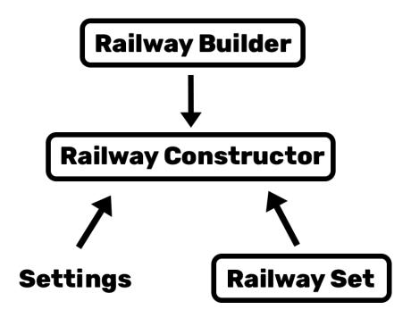
**Railway Constructor:** This component is the heart of the system, it holds both the construction settings and a reference to a Railway Set.
