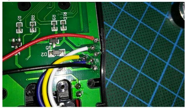
To get the cases of both devices closed i cut small notche in each case for the wires and closed both cases up. As a last step I hot glued them together with a piece of plastic in the back for more strength (be carefully not to glue shut one of the two batteries compartments)
