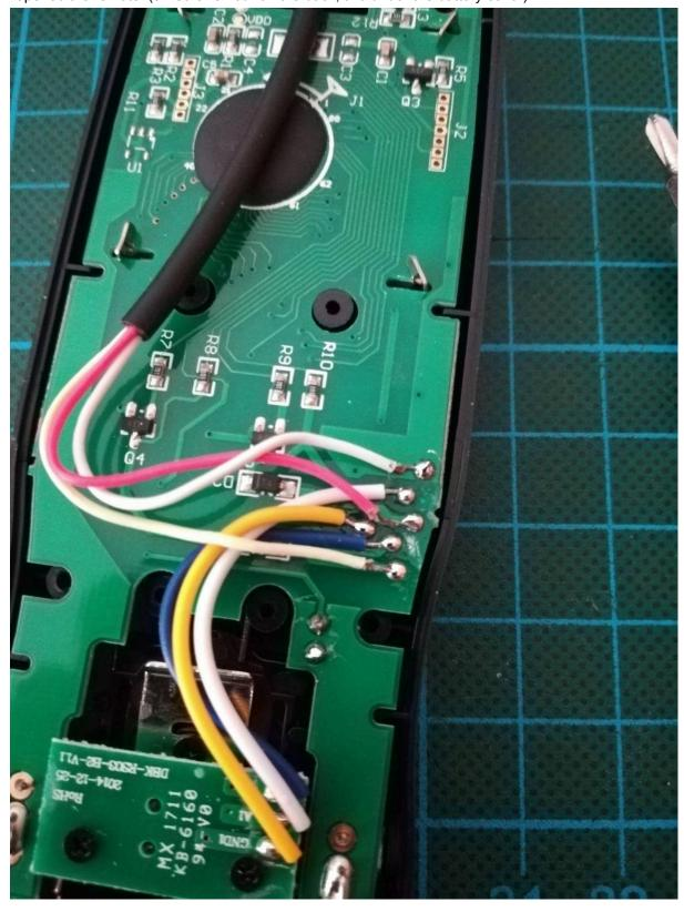
Now I desoldered the three wires from the big black external cable and just removed it completely. The two wires from the Bluetooth remote were soldered to two of the now empty pads like shown in the picture below.
