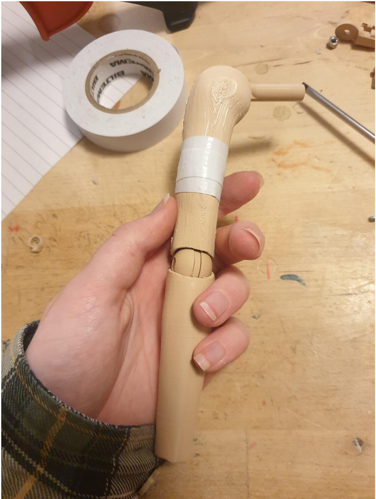
Assemble wrist 1 and 2 with a 8mm bolt.
