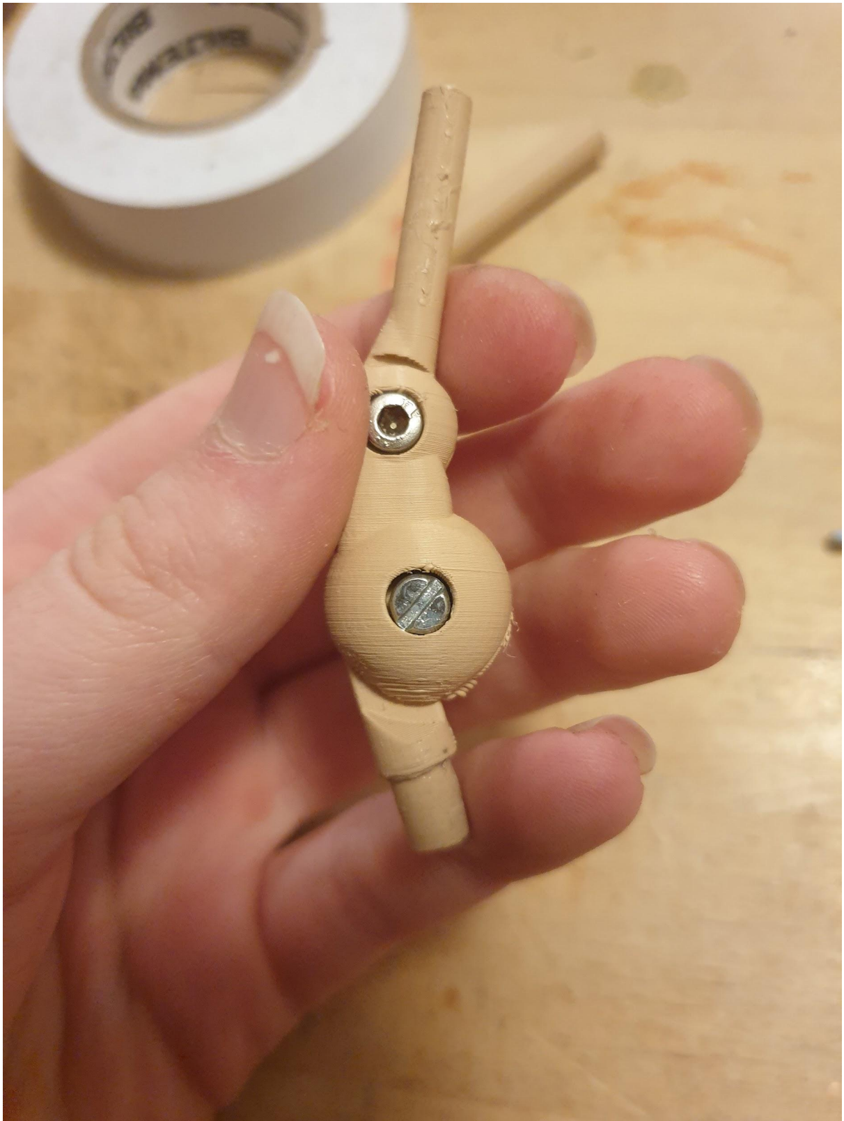
Slot it into the lower arm bone. I glued this in place as well.
