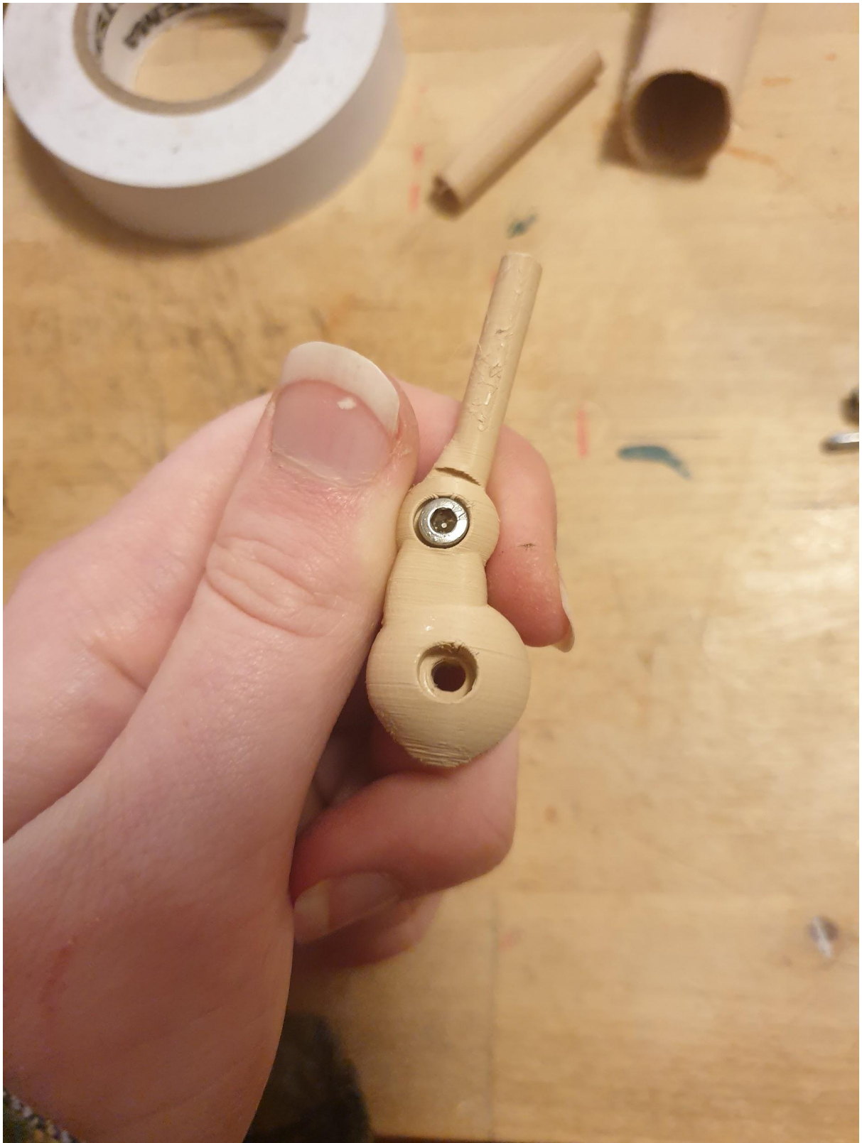
And elbow lower with a 15mm bolt.
