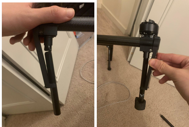
Figure 1 Before and after the leg replacement
