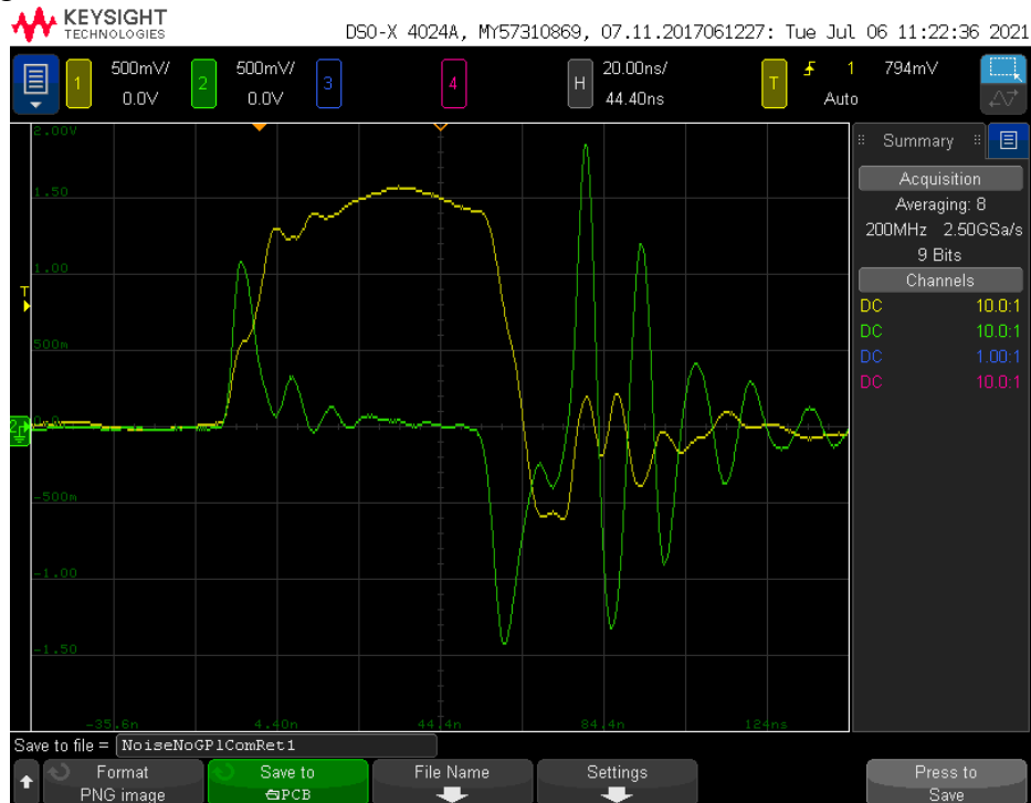
Figure 2.) Yellow signal is the voltage measured at the 47 \Omega resistor (TP4) and green signal is the voltage of the victim line (TP5). Both vertical scales are 500mV/div. and the vertical time scale is 20nsec/div.
