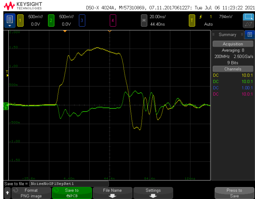
Figure 3.) Yellow signal is the voltage measured at the 47 \Omega resistor (TP4) and green signal is the voltage of the victim line (TP5). Both vertical scales are 500mV/div. and the vertical time scale is 20nsec/div
