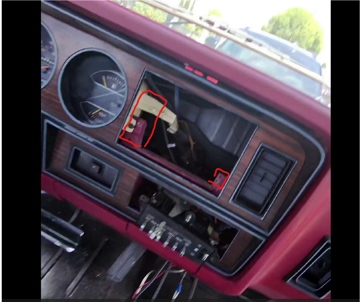
Red boxes indicate the two small trim areas: dash frame and instrument cluster arm
