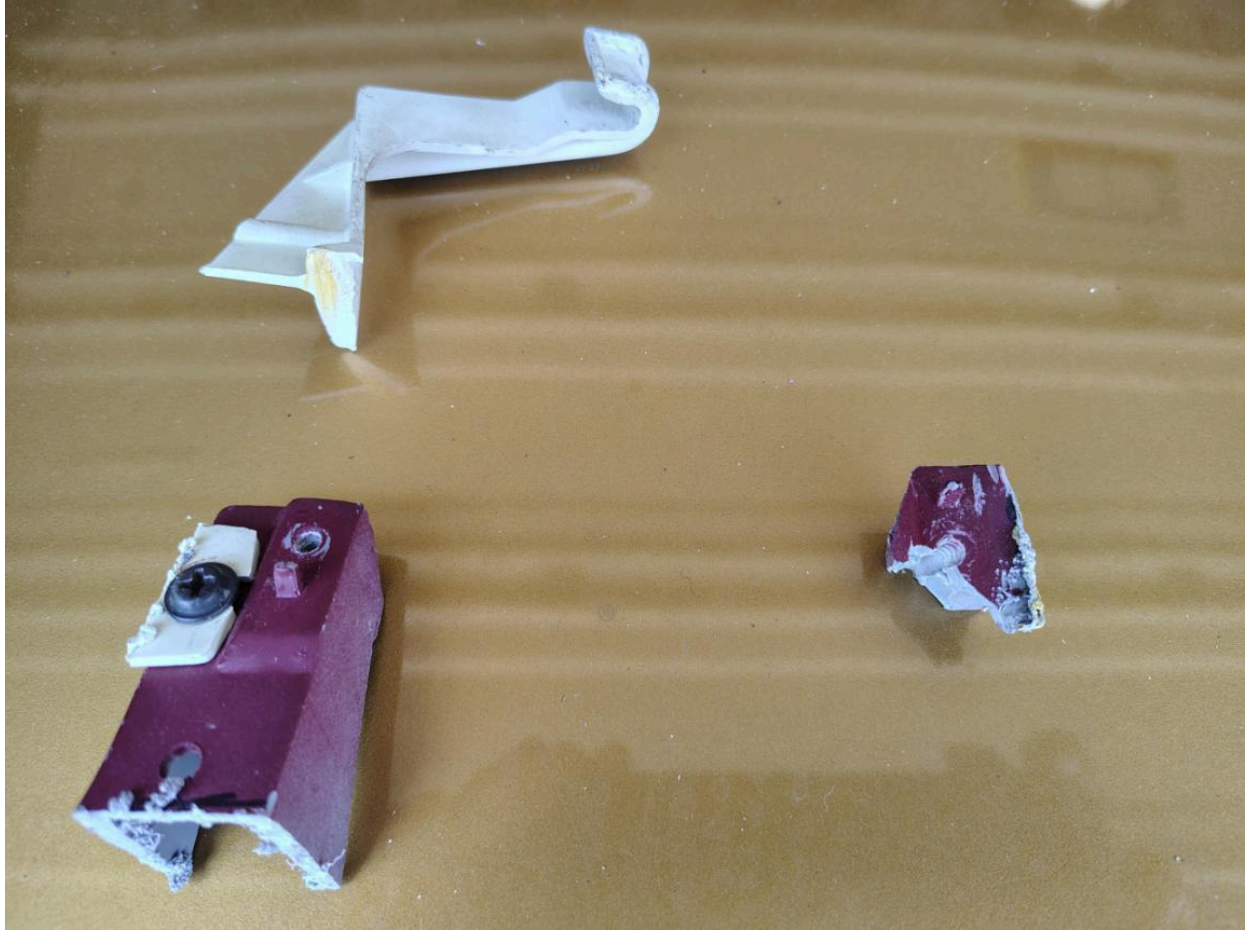
The three small pieces removed: instrument cluster arm bracket (top) and two dash frame sections (bottom)
