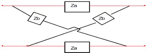
**Q.44.** Find the h parameters of the circuit shown in figure.
