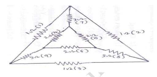
**Q38.** Draw the graph for the network shown in figure below. Write the cut-set schedule & obtain equilibrium equations and hence calculate values of branch voltages and branch currents
