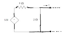
Q30. Write the statements of Thevenin's and Norton's theorem and also write the limitations. Q31. Find the current in 2 Ohm resistance resistance in the network shown in Fig. (I). (using Norton's theorem)
