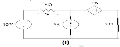
Q32. Write the complete and reduced incidence matrix for given graph a network.
