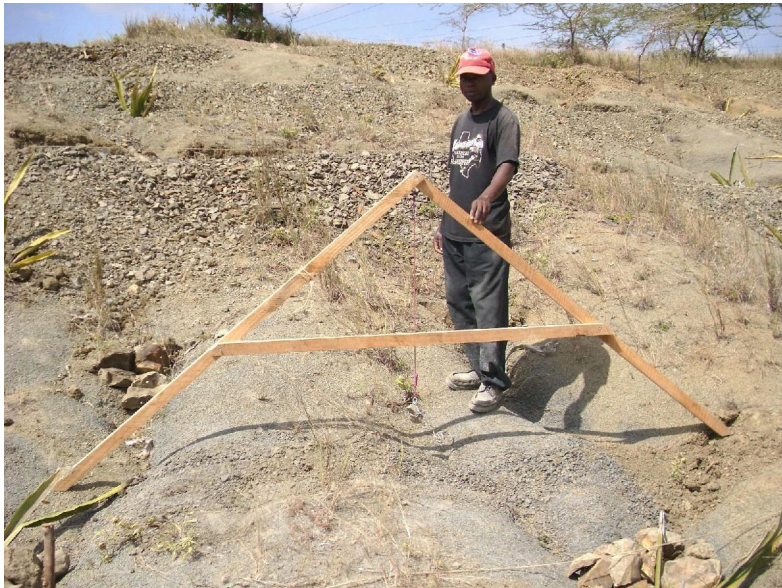
Picture 3: The use of an A-frame to identify the contour line
