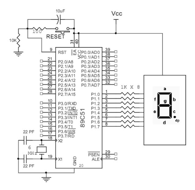
o Except 7 segment display interfacing, this circuit diagram shows minimum interfacing required for microcontroller to operate. That is, Reset circuit, Crystal oscillator, Vcc=5V, GND & EA' Pin.
