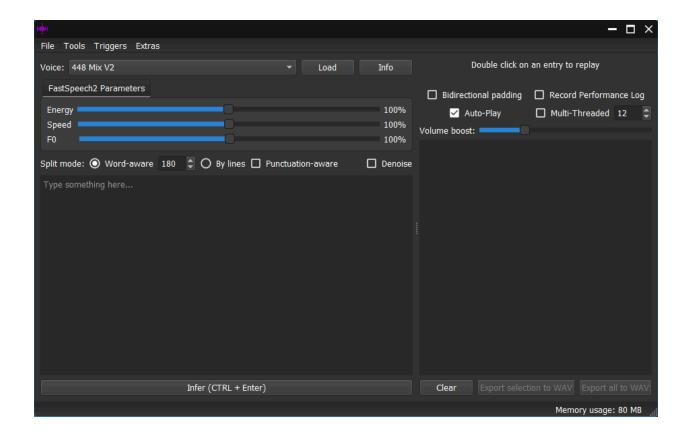
To start, click the dropdown menu next to *Voice* and select one (or keep it as is) and click **Load** to load the model. Note that for every loaded model the program uses 500MB of RAM idle. Also, you don't have to explicitly load the model, clicking the **Infer** button without a loaded model will automatically load it first. If the model is a multispeaker one, once you click Load, the list of speakers will appear.
