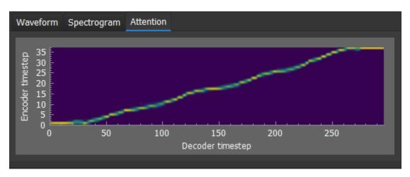
Only available in Tacotron2, the attention plot shows how the model managed to align the generation. The closer to a nice, diagonal line, the better.
