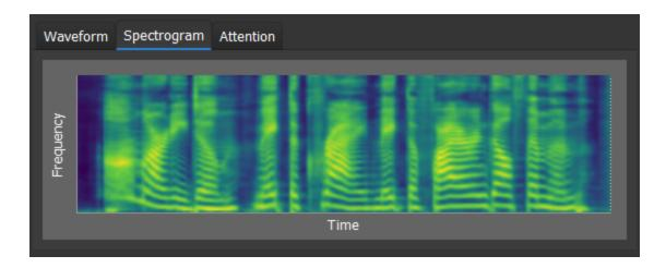
Direct from the Text2Mel model's outputs, the spectrogram is a data-dense representation of sound as perceived by the human ear, and more detailed.
