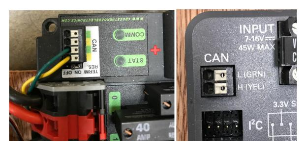
The CAN bus wires are yellow and green 22 AWG wires. The green wire serves as a ground wire.
