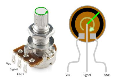
Potentiometers are a type of absolute rotary sensor that uses resistance to track the physical property position. Ring a bell? This is an analog sensor, since by varying resistance, it in turn varies voltage. How does the potentiometer accomplish this?
