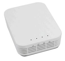
In order to power the radio, \_\_AWG wire must be routed from the 12V/2A port on the VRM in order to power the radio using a PoE injector cable, which plugs-in to the 18-24vPOE port on the radio and the male end of an ethernet cable routed to the roboRIO. This is illustrated below. PoE stands for Power over Ethernet. This is a passive cable that combines the electrical current of both the power and signal wiring, which would normally stand alone.
