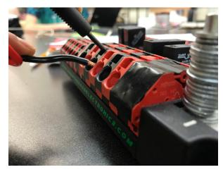
You must insert the wire while holding the screwdriver firmly down. This will take trial and error, as the screwdriver slips easily, but comes with practice.
