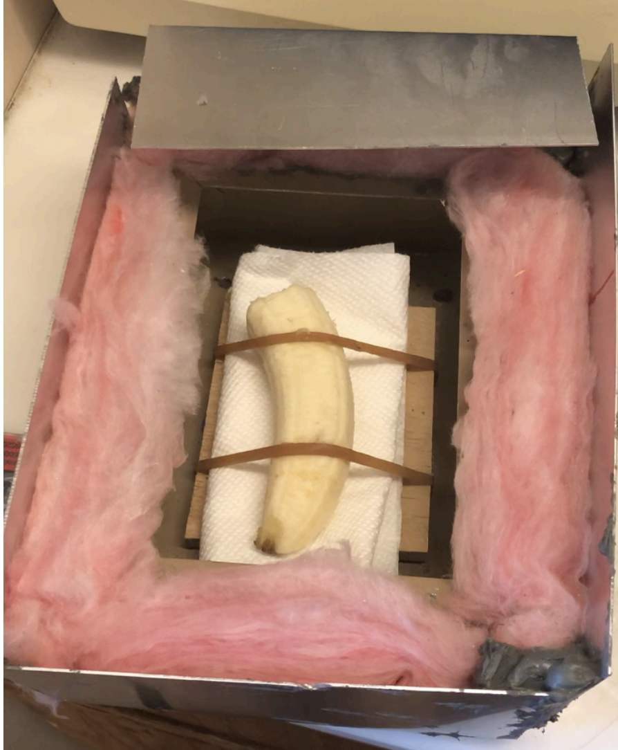
Figure 12, Depicts the fully constructed Black Box with the test subject prior to being placed in the oven at 200 degrees Fahrenheit. Notice the individual layers of aluminum, insulation, and another aluminum box as well as the corners sealed with fireplace caulk.
