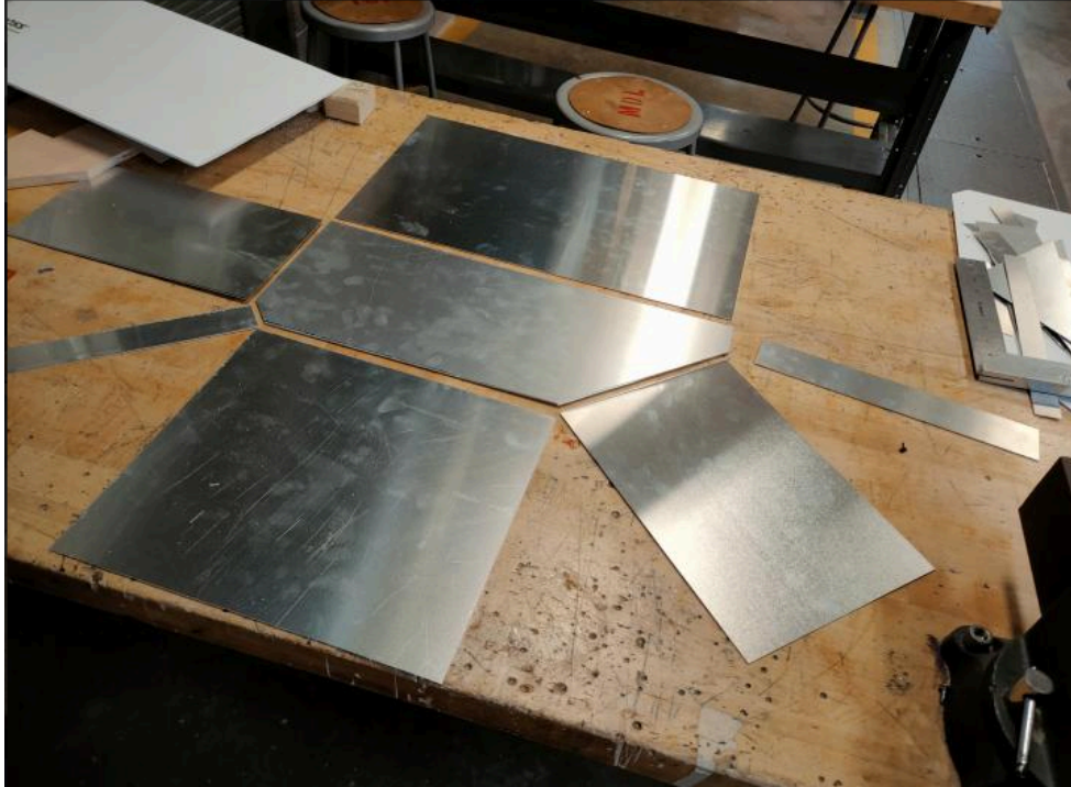
Figure 38, Faces of the frame cut
