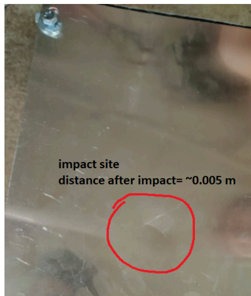
Figure 48, Impact site after the test
