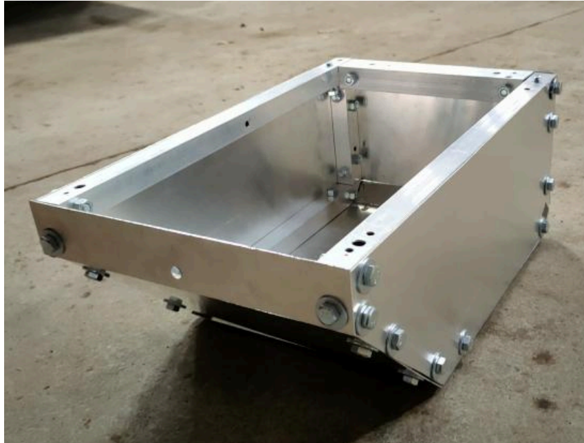
Figure 36, Frame with holes drilled on the front
