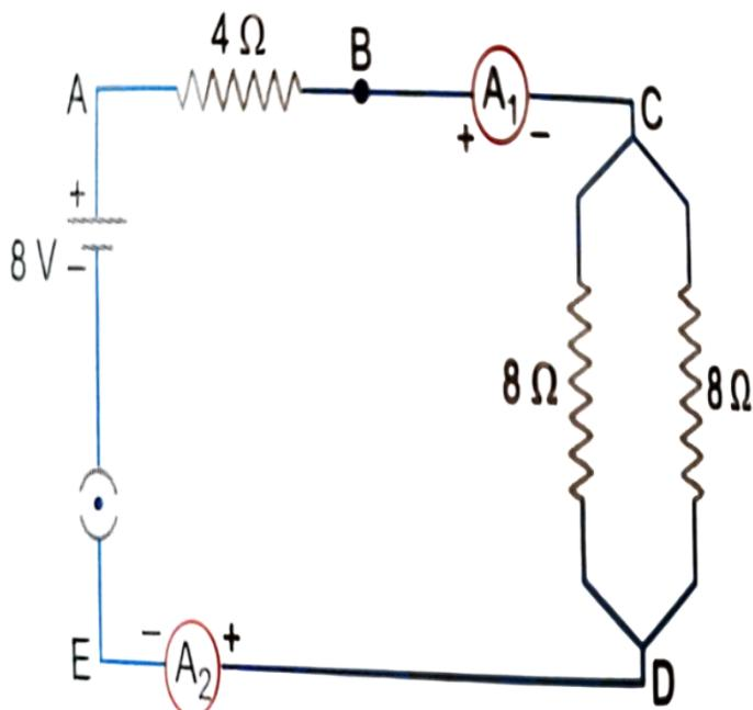
Find out the following in the electric circuit given in the figure-
