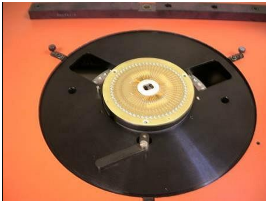
Figure 17 - Probe Card in the Cover With the Tips Up
