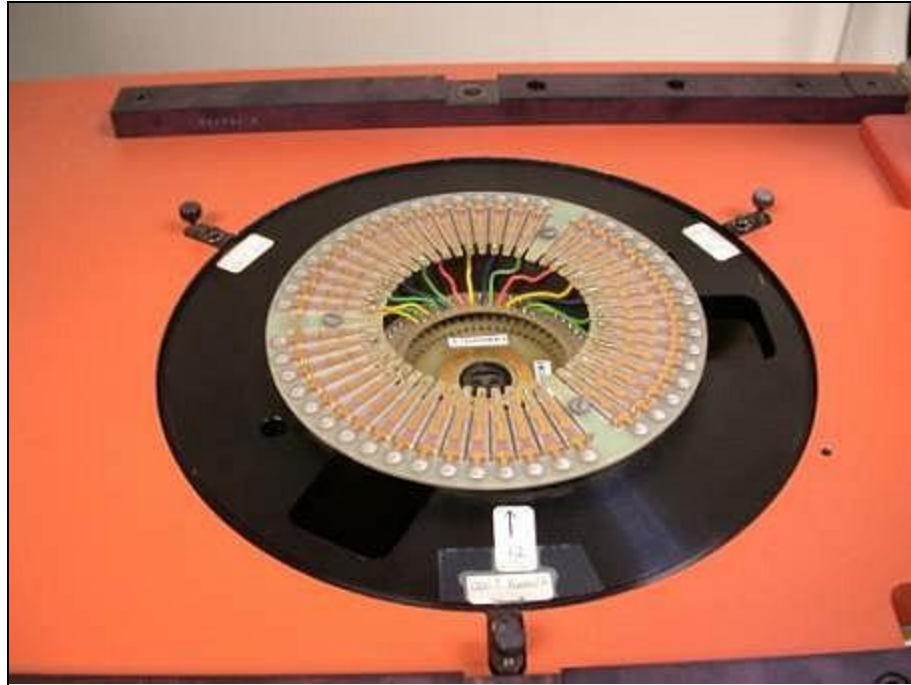
Figure 16 - Probe Card in the Cover With the Tips Down
