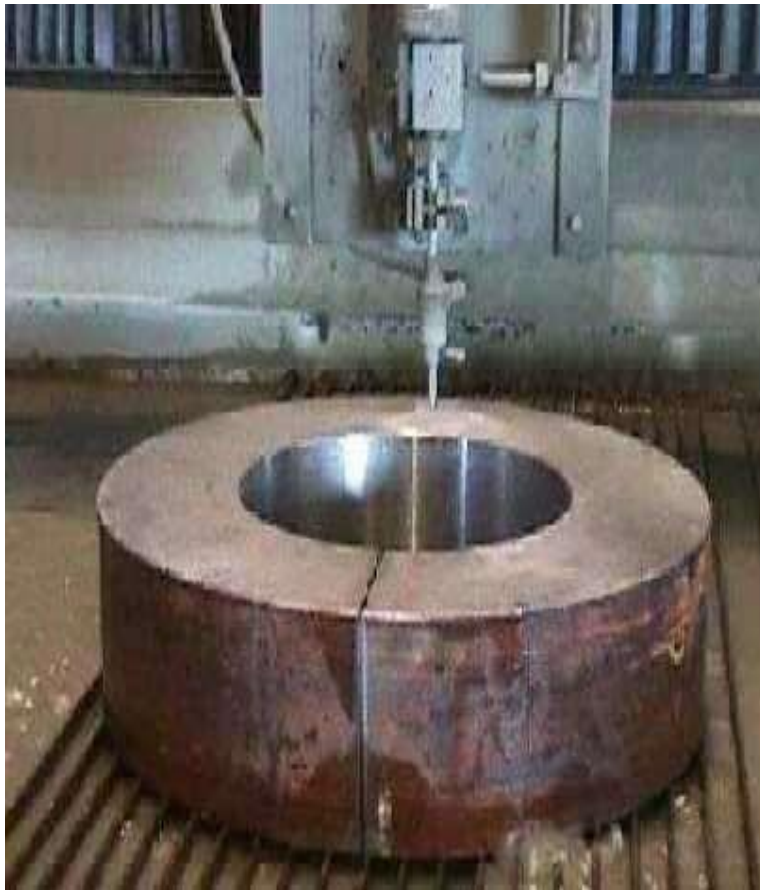
Abrasive water jet cutting
