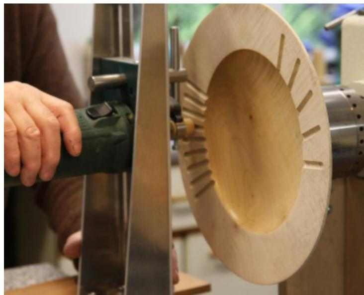
The jig is positioned with the clamped router in such a way that the guide bush touches the workpiece. In order to carry out the milling at the desired position, the apparatus is moved accordingly.
