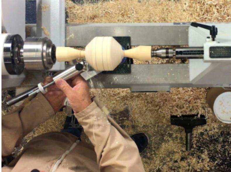
The standard jig fits onto most flatbed bars. We also have the adaptor for round bar lathe beds.
