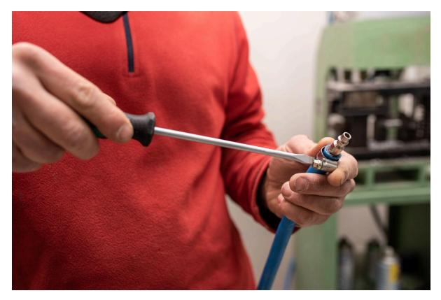
alt: A technician makes a precise, incremental adjustment to a hydraulic fitting with a screwdriver, demonstrating a key step in setting a flow control valve.
