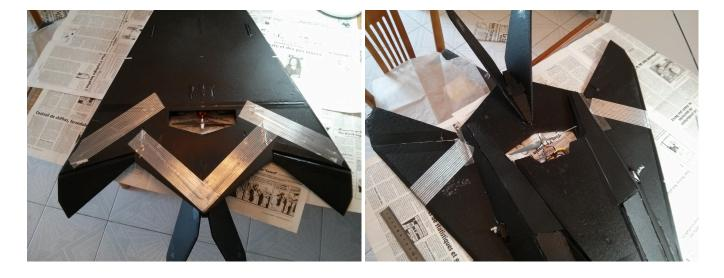
And finally, I reinforced the trailing edges of the tails but I'm not sure if this will do any good.
