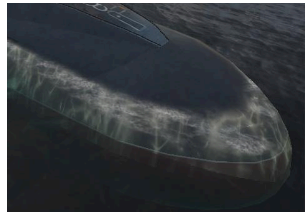
Normals reconstructed from the depth texture. The gradient gets quantized.
