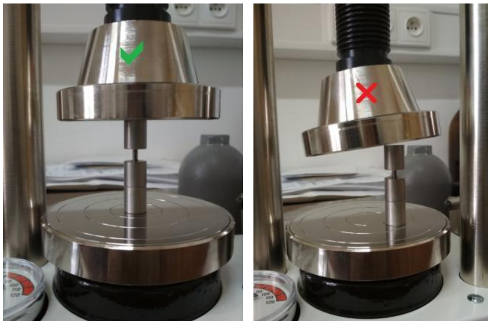
Figure 2.7: Press mold correctly (left) and wrong (right) inserted into the press
