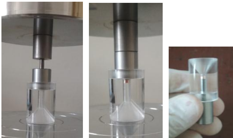
Figure 2.10: Extrusion of a tablet from a compression mold
