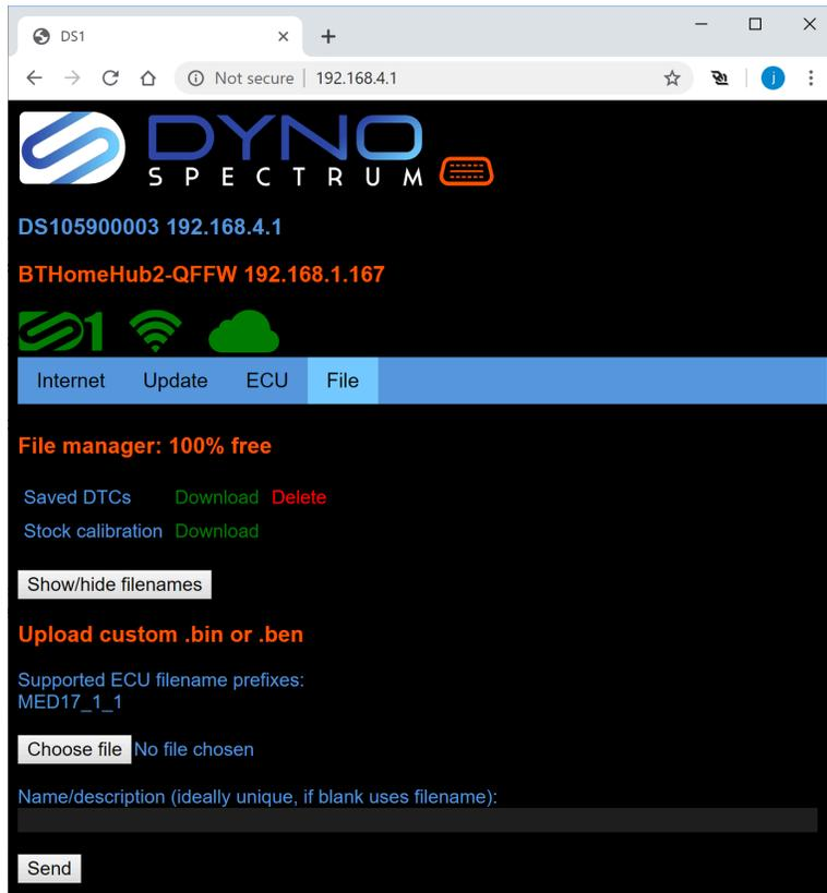
Here you can download the stock calibration for use in TunerProRT for normal or realtime tuning. The xdf definition is also available to download (not shown here) as a zip which must then be unzipped to use with TunerProRT.
