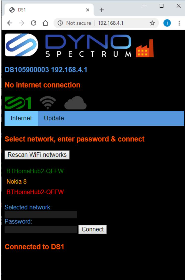
The three networks here are shown coloured according to signal strength, green, yellow or red. Here, the green access point is 10 feet away, the yellow hotspot from a cell phone is 50 feet away, and the red access point is 70 feet away through two brick walls and is too weak to use reliably.
