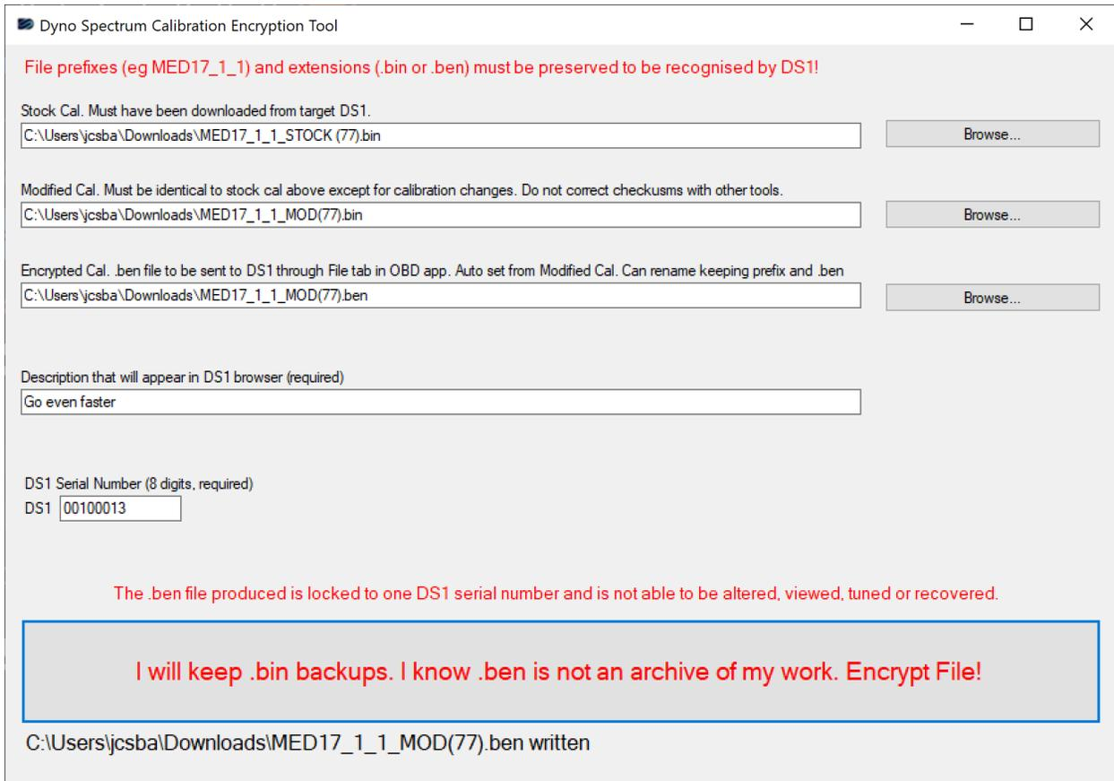
When the .ben file is sent to the DS1 through its File tab, the description used is the one that was entered in the Encryption tool. Prefix must be MED17\_1\_1 for our initial supported ECU, and extension must be .ben
