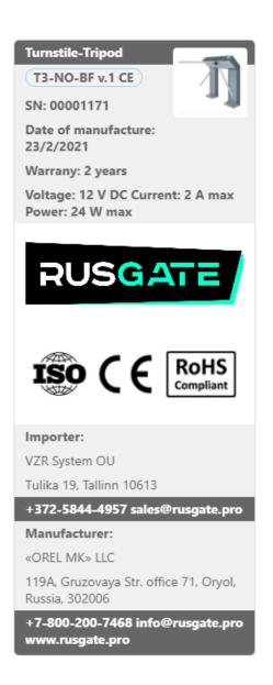
Turnstiles have physical marking in the form of laminated, moisture-resistant labels located under the front casing. To read information from the label, it is necessary to remove the front casing (pos. 2), having previously disconnected the barrier arms. The label is as follows:
