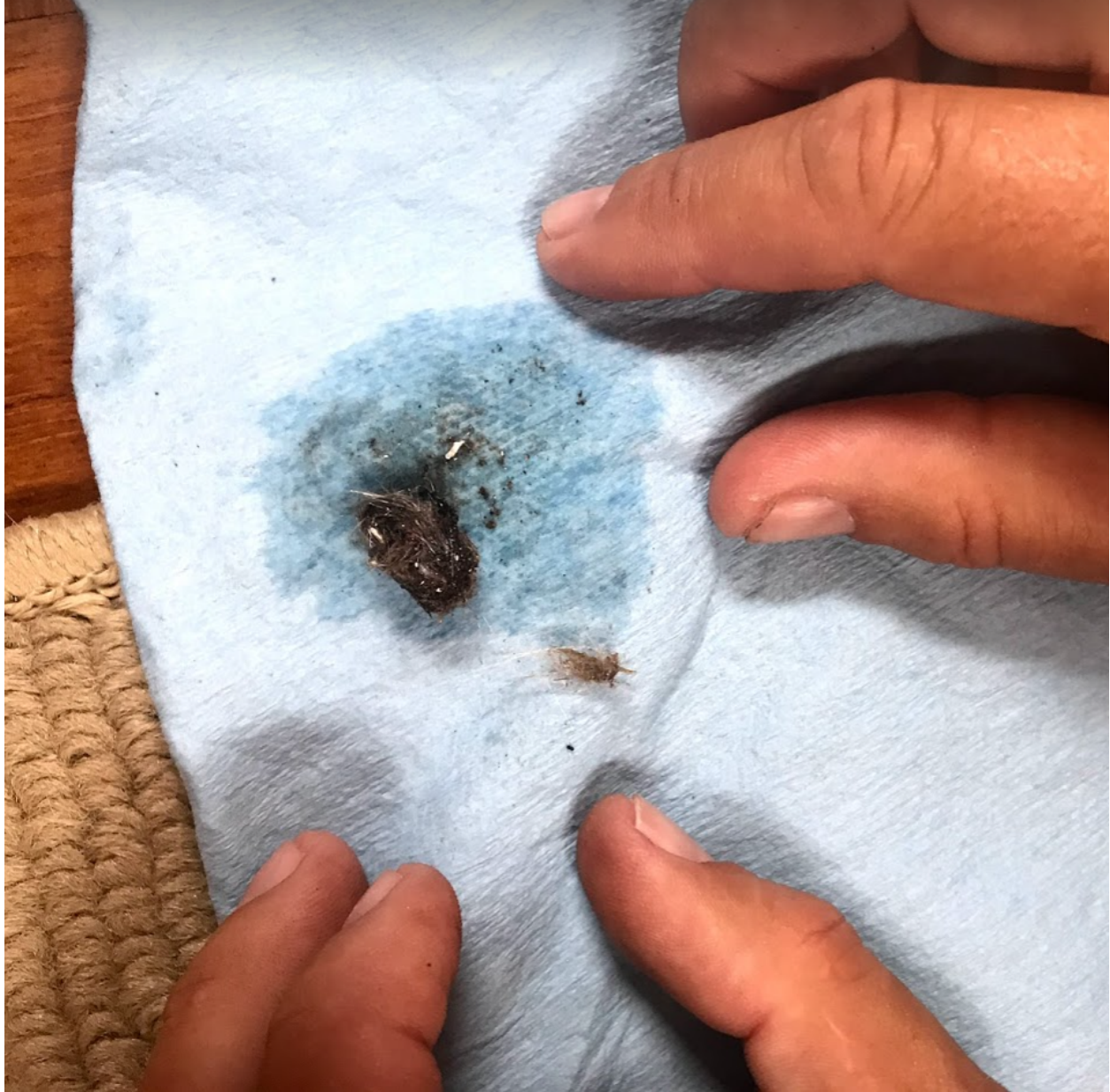
This is what came out of the valve when we used the dinghy pump to force it out. Fibreglass strands and some dirt.
