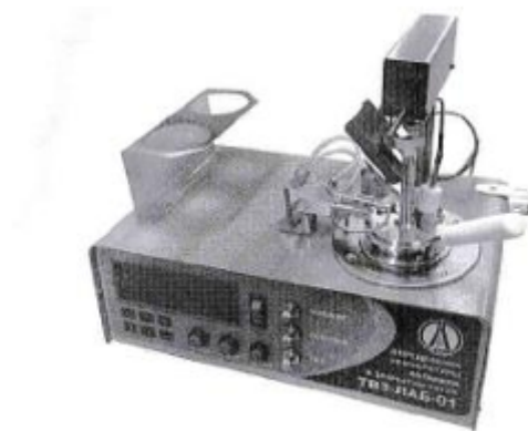
Figure 2. Apparatus for determining the flash point of oils in a closed cup
