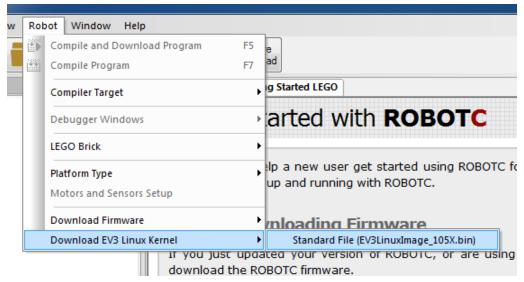
B: The "Entering Kernel Firmware Download Mode" is when the EV3 is switching from "run" mode to "bootload" mode. This may take 5-10 seconds to switch. If you get an error message from this point, simply try the upgrade again and it should be successful.
