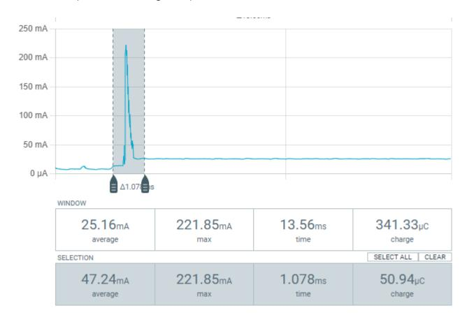
The effect of using the ON/OFF pin (basically power off, doesn't seem to save inrush on re-enable)
