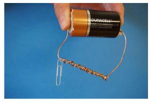
Then the students tested whether or not the size of the battery had an effect on the number of paperclips the electromagnet could attract. Students used a *9V battery*, and a *AA battery*.
