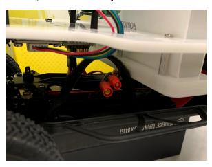
2. Plug in a car battery. Make sure the battery is plugged in all the way. (You have to press pretty hard for this to happen.)
