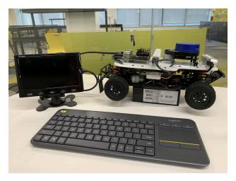
3. Plug in battery (Jetson power into the port with two thunderbolts)
