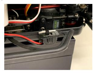
You should hear a beep. If you do not hear a beep, make sure the battery you are using is charged. (Plug it in until the light turns green.)
