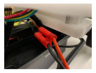
3. Put the battery under the velcro to secure it.
