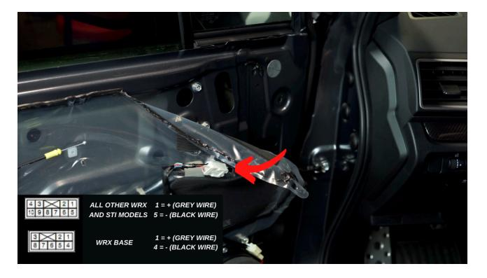
Note that the harness is marked "L" and "R" to designate the left (drivers side) and right (passenger side) harnesses.
