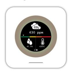
Regular mode is the default mode that is active when you first turn on the device. It displays the CO<sub>2</sub> level, temperature, humidity, and battery level on the screen in real-time without any alarms.
