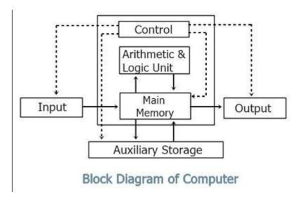
In the above diagram, both control (control unit or CU) and arithmetic & logic unit (ALU) combinely called as Central Processing Unit (CPU).
