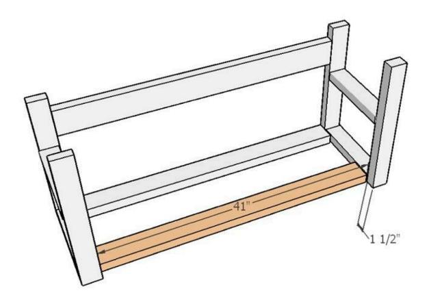
**Step 11.** Attach 2x4s sized 9 ½" brace into the bottom bench with glue and screws.
