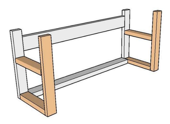
**Step 10.** Attach 2x4s sized 41" into bottom bench with glue and 2  $\frac{1}{2}$ " screws. Make sure that this 2×4 41" needs to be inset 1  $\frac{1}{2}$ " from bench outside part.
