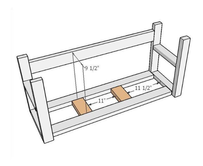
**Step 12.** Attach 1x8s sized 48" into bottom bench with glue and wood screws.
