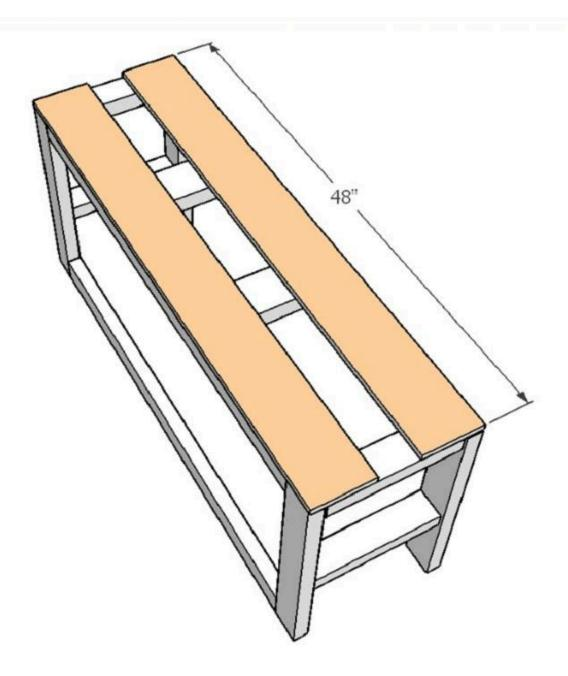
**Step 13.** Attach 1x3s sized 48" into bottom bench with glue and wood screws. Make sure that there is  $\frac{1}{4}$ " gap between each board.
