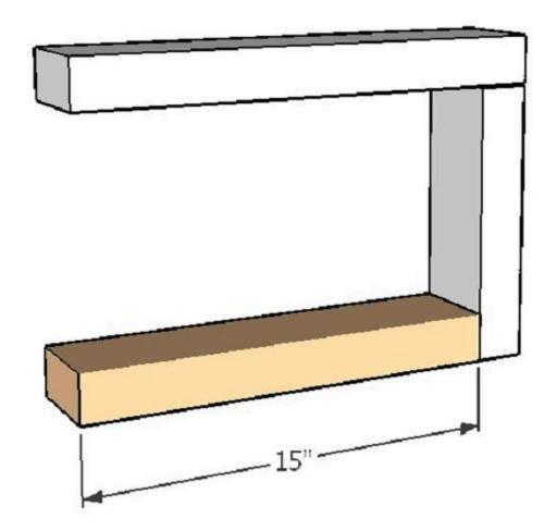
**Step 4**. Attach two bench arms into top bench back support. Make pre-drill holes using 1 ½" Kreg jig. Then, secure all pieces using glue and 2 ½" screws.
