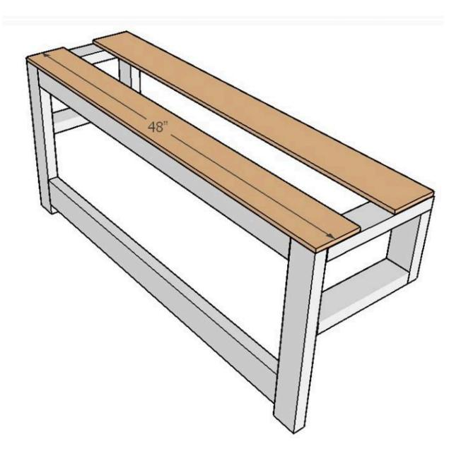
**Step 6.** After the seat support sides are set, insert the middle piece from  $1\times3$  (48") with wood glue and screws. Make sure to leave  $\frac{1}{4}$ " space between the top bench boards.
