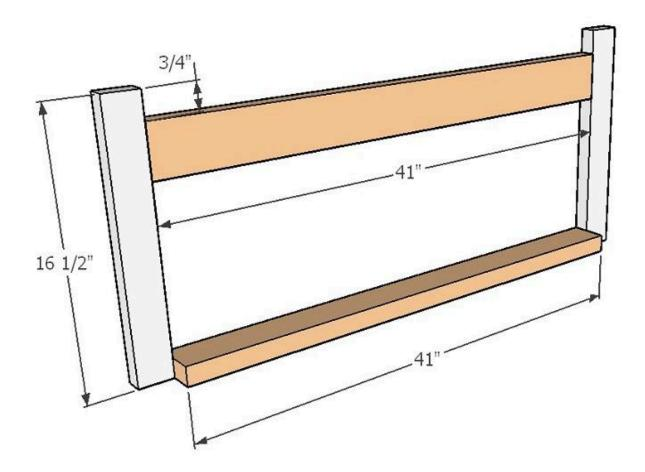
**Step 8.** Build the side arms of bottom half. Attach top side and front side braces into 2x4s sized 17 ¼". Secure the joint using wood glue and 2 ½" screws. Build two side arms!
