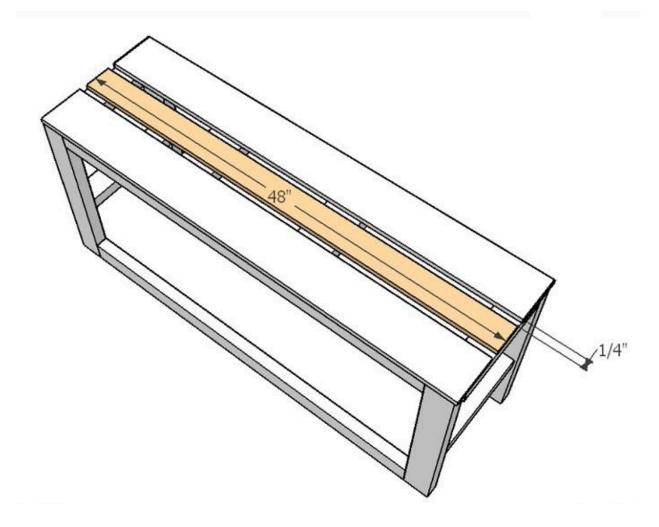
**Step 14.** Build the backs for the convertible bench. You can add some hardware to join the top and the bottom parts of the bench altogether.
