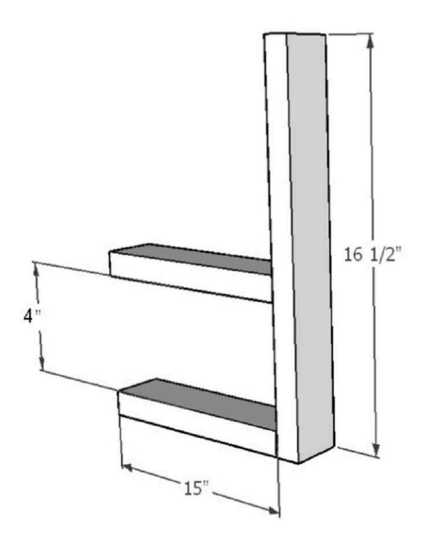
**Step 9.** Attach two side arms into bottom back support. Secure the joint using glue and 2 ½" screws.
