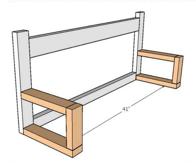
**Step 5.** Then, attach two pieces of  $1\times8$  (48") seat supports onto the top bench with wood glue and wood screws or brad nails. These two pieces should be in line with the bench outside parts.
