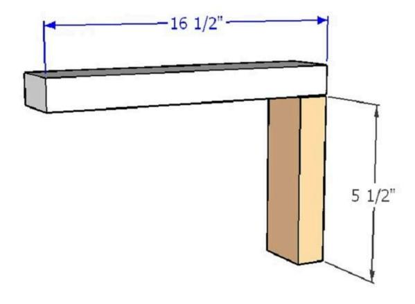
**Step 3.** Insert the bottom side braces from  $2\times4$  boards sized 15'' into the side arm frame. Make some  $1 \frac{1}{2}$ " pocket holes to connect the brace. Attach the bottom brace using glue and  $2 \frac{1}{2}$ " screws. Use the same method for both bench arms.
