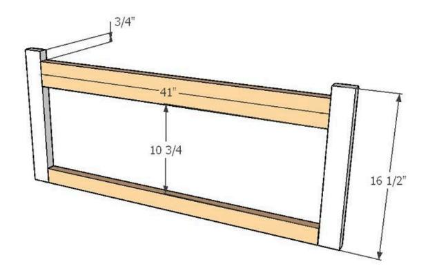
**Step 2.** Build the side arms from mounting the top and front side braces. The top side is  $2\times4$  brace with  $16\frac{1}{2}$ " and the front side is  $2\times4$  brace with  $5\frac{1}{2}$ ". Make pre-drill holes using  $1\frac{1}{2}$ " Kreg jig setting. Then, attach all braces using glue and  $2\frac{1}{2}$ " screws. Apply the same step for building one more bench side arm.
