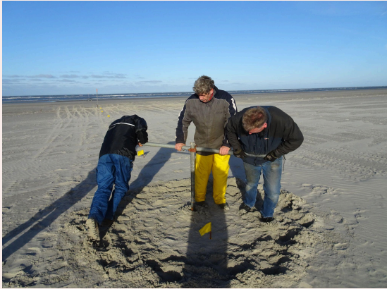
Picture 1: Anchoring the instruments in the sand was hard work. The poles needed to be driven into the sand at least 2 m to prevent them from falling during the inundation of the island.
