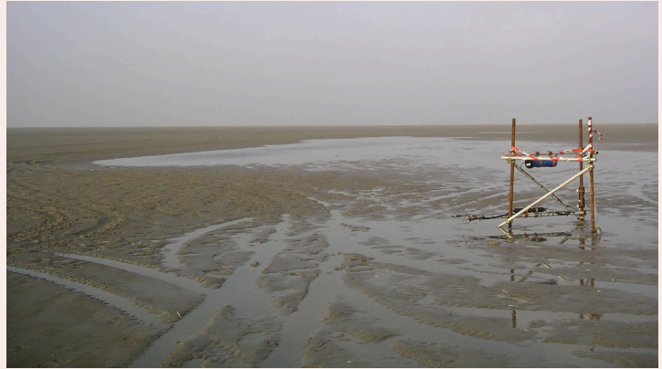
Picture 2: The frame was equipped with instruments measuring waves and currents
