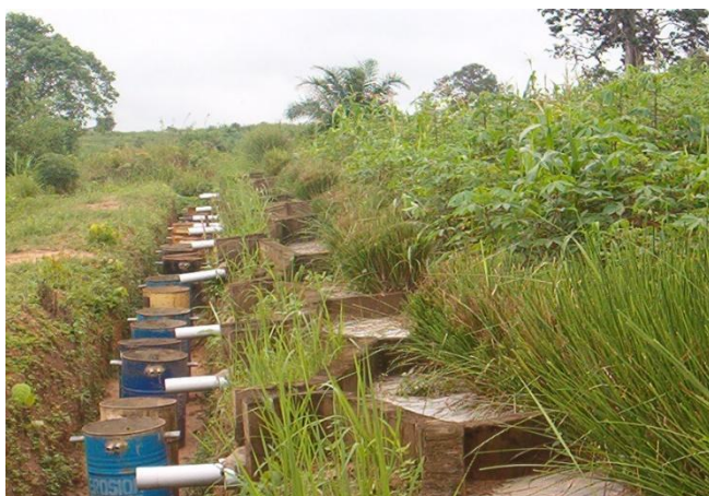
Plate.4: Sedimentation drums installed in the ground in a trench dug at the foot end of the erosion plot with vetiver buffer grass strips at lower slope.
