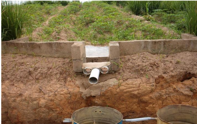
Plate 2: End of 50 m long erosion plot with a funnel neck end fitted with multi-slots (3 outlet divisors) PVC pipes to direct \frac{1}{3} of runoff and soil loss (sediment flow) into the sedimentation drum under Usual Practice plot.
